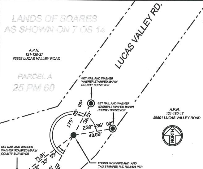
7 OS 14 REPLACED WITH STANDARD COUNTY MONUMENT PER UNIFORM CONSTRUCTION STANDARDS DRAWING #300
